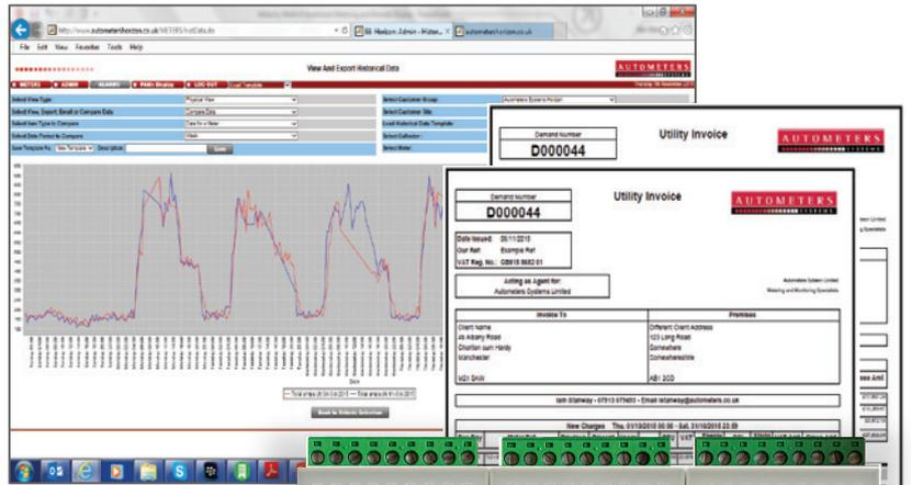
RS 485 Modbus Communication to enable full data retrieval of kWh for Graphic analysis and Billing
