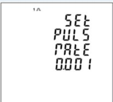
Pulse rate options: 0.001 , 0.01 , 0.1 , 1, 10, 100, 1000 kWh / kVarh per Pulse
