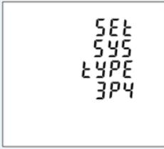
The screen shows the currently selected power supply is three phase four wire
