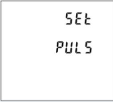
This option sets the pulse output type, pulse rate, duration time.
