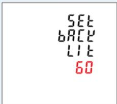
The meter provides a function to set the time the back light is on. Options: ON/OFF/5/10/30/60/120 minutes. Default: 60
