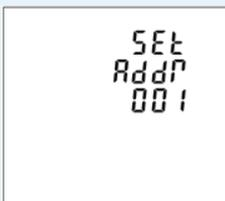
An RS485 network can accommodate up to 255 different devices, each identified by an individual address.
