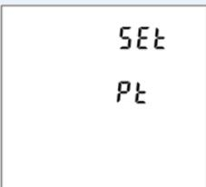
The meter has been designed to work in 3 phase 4 wire or a 3 phase 3 wire network and this requires a primary and secondary voltage ratio input. The default is a 3 phase 4 wire configuration.
