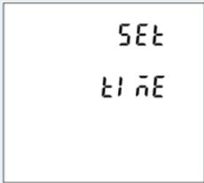
This option sets the backlight on time and display scroll time.
