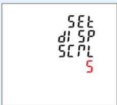
The meter provides a function to set the Display scroll time. Options: 1~255s. Default: 5
