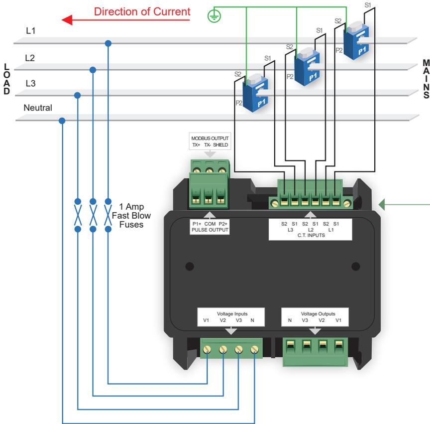
The back of the meter shows the green connections where the cables must be wired into, each separate green connector is a plug and socket.
