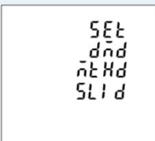
The screen shows the Demand calculation method: Fixed interval time or Sliding window.
