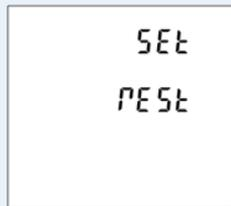
This unit provides a function with reset for Energy and Demand, and all parameters.
