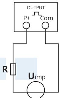
ATTENTION: Pulse output must be fed as shown in the wiring diagram below. Scrupulously respect polarities and the connection mode. Opto-coupler with potential-free SPST-No Contact.
