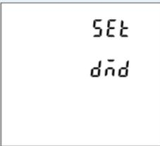
This sets the period in minutes over which the current and power readings are integrated for maximum demand measurement.
