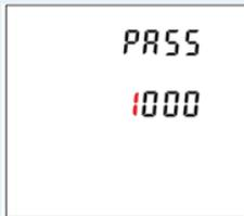
Setting-up mode is password protected, so you must enter the correct password.
