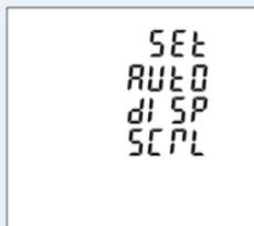
This meter provides a function with automatic display scroll setting.
