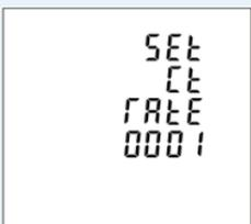
To set the primary current ratio in the meter you must program the divider into the meter. e.g. to set 200/5 amp input "0040" (Divide the primary by 5) 5 amp being the secondary of the c.t. see section 4.3.3 for the table.
