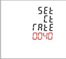
Example of how the display should look for a meter programmed to 200/5 amp. See table for more settings.
