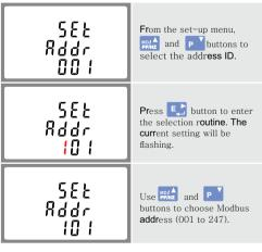
On completion of the entry procedure, press button to confirm the setting and press button to return the main set-up menu.
