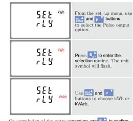
On completion of the entry procedure, pre: to confirm the setting and press V/A to return to the main set up menu.
