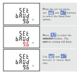
On completion of the entry procedure, press to confirm the setting and press  $V_{ESC}^{VA}$  to return to the main set up menu.
