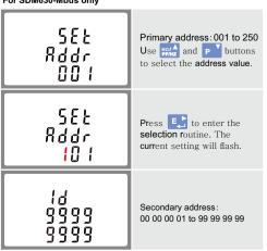
On completion of the entry procedure, press to confirm the setting and press  $\bigvee_{ESC}^{V/A}$  to return to the main set up menu.
