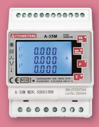
This unit can be powered from a separate auxiliary (AC or DC) supply. Alternatively it can be powered from the monitored supply by linking the voltage reference and neutral reference in to terminals 5 + 6 (Please refer to wiring diagram).
