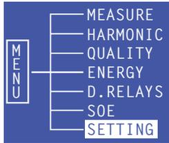
There is a security level here which must be entered to allow you to program the meter. The default password is "0001"
