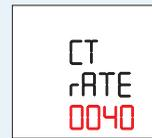
Example of how the display should look for a meter programmed to 200/5 amp.
