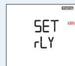
From the set-up menu, use **MD** and **P** buttons to select the Pulse output option.
