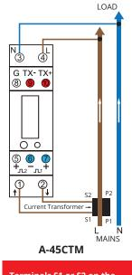
Terminals S1 or S2 on the current transformer or the meter must not be common to Earth
