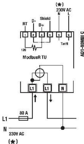
Terminals 5 & 6 only require 230 Volt from an external time switch when using more than one tariff.
