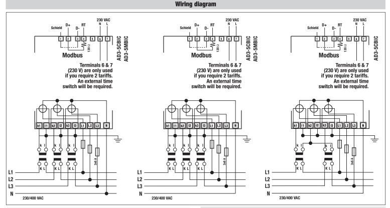
(N) Neutral wire must be connected the meter
