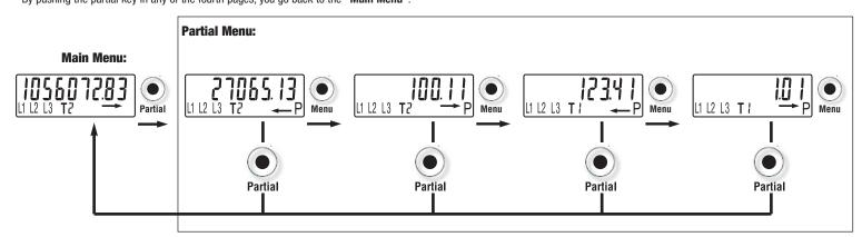
A pressure of 4 sec. of the "Menu key", in every page of the "Partial Counters" allows to enter in the zeroing menu of the "Partial Counters", and on the display appears "rESET".
