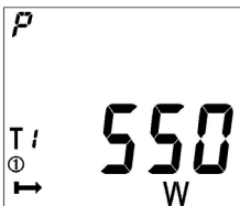
Current total active power 550W
