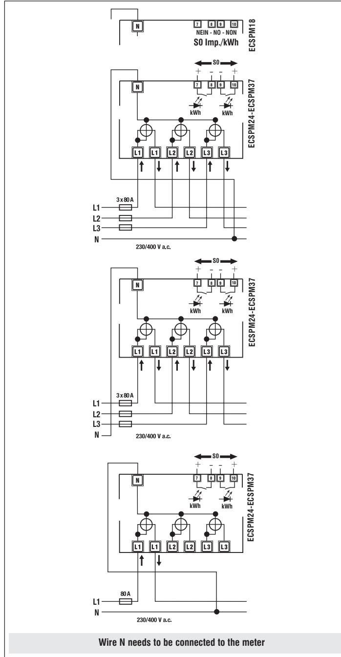
A fuse of 80 A is recommended for the line protection.
