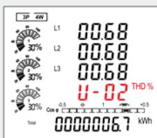
Press the button
