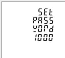
This meter provides a function with password setting.
