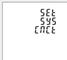
This meter provides a function where you can adjust the current transformer connection internally via the front keys. Each phase can be altered.
