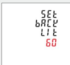
The meter provides a function to set the time the back light is on.
