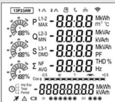
The first screen lights all LED segments and can be used as a display LED check
