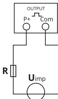
ATTENTION: Pulse output must be fed as shown in the wiring diagram below. Scrupulously respect polarities and the connection mode. Opto-coupler with potential-free SPST-No Contact.
