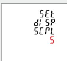
The meter provides a function to set the Display scroll time.
