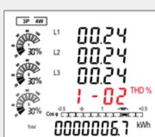
Press the button
