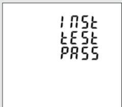
The unit performs a self-test and the screen indicates if the test is passed.
