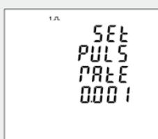
Pulse rate options: 0.001 , 0.01 , 0.1 , 1, 10, 100, 1000 kWh / kVarh per Pulse
