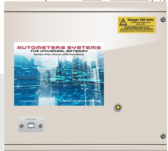
The AUG is a surface mounted GPRS enabled data collection device capable of storing information from up to 350 meters via 3 separate Lans
