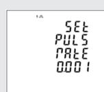
Pulse rate options: 0.001, 0.01, 0.1, 1, 10, 100, 1000 kWh / kVarh per Pulse. Default: 0.01 kWh (100imp/kWh)
