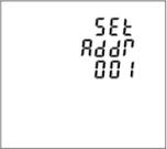
An RS485 network can accommodate up to 255 different devices, each identified by an individual address. The Modbus address range on the HT-35 is between 001~247
