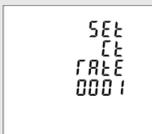
To set the primary current ratio in the meter you must program the divider into the meter. e.g. to set 200/5 amp input "0040" (Divide the primary by 5) 5 amp being the secondary of the c.t. See table below. Options: 1~2000. Default CT rate 1. (New Ratio Must Be Programmed Into The Meter)
