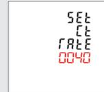
Example of how the display should look for a meter programmed to 200/5 amp. See table for more settings.
