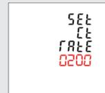
Example of how the display should look for a meter programmed to 200/1 amp. See table for more settings.
