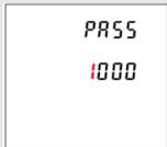
Setting-up mode is password protected, so you must enter the correct password.
