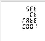
To set the primary current ratio in the meter you must program the primary current ratio into the meter. e.g. to set 200 amp input "0200"
