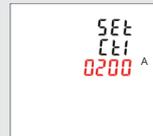
Example of how the display should look for a meter programmed to 200 amp.
